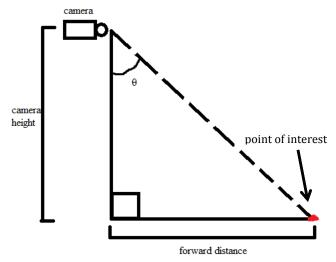
forward distance and the tangent of the horizontal angle of the particular pixel of the camera. The distances of these points are then sent to the SLAM component to be mapped as obstacles.
